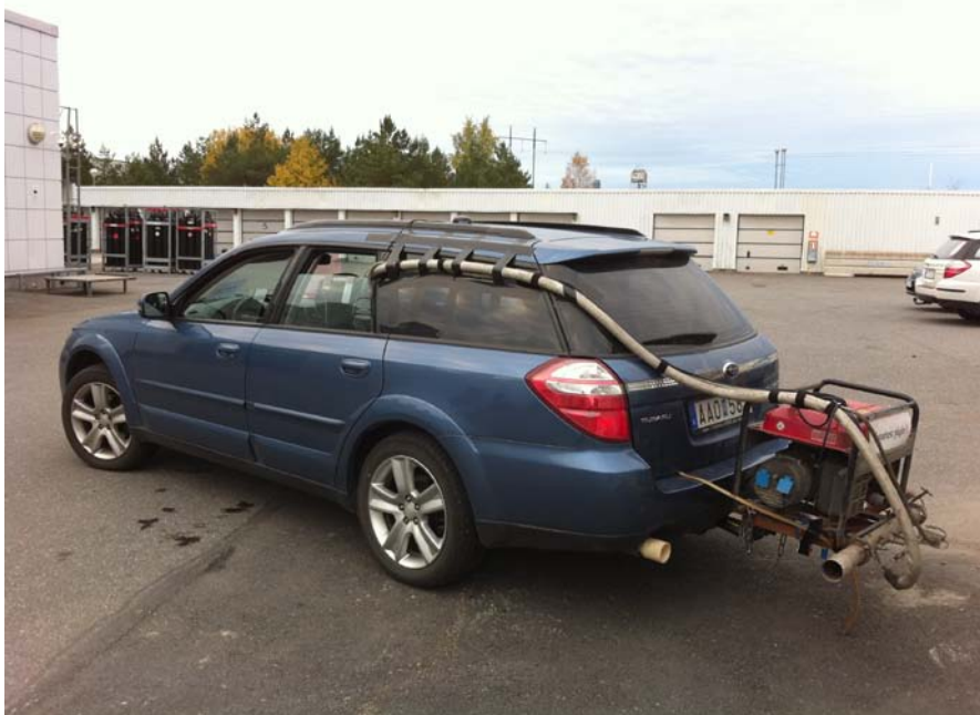
Figure 1: Subaru Legacy with PEMS test equipment,
