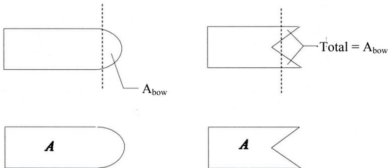
**Figure 4.4.1: Plan view of two different craft styles**
