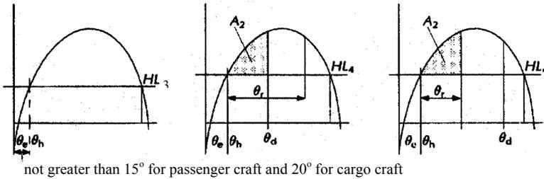
Figure 2 - Damage stability
