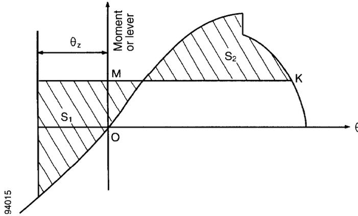
Figure 1 – Static stability curve
