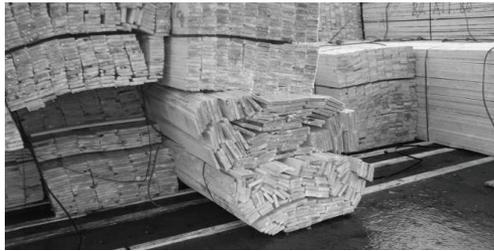
**Figure 6.2. Example of poor rigidity**
