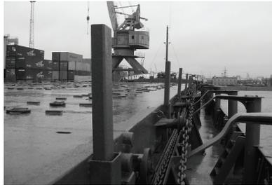
**Figure 6.7. Example of uprights for bottom blocking**
